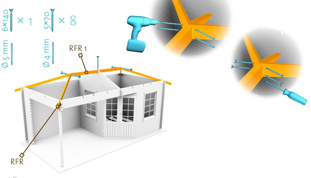
INSTALL THE ROOF PURLINS AND ATTACH THEM WITH SCREWS.
