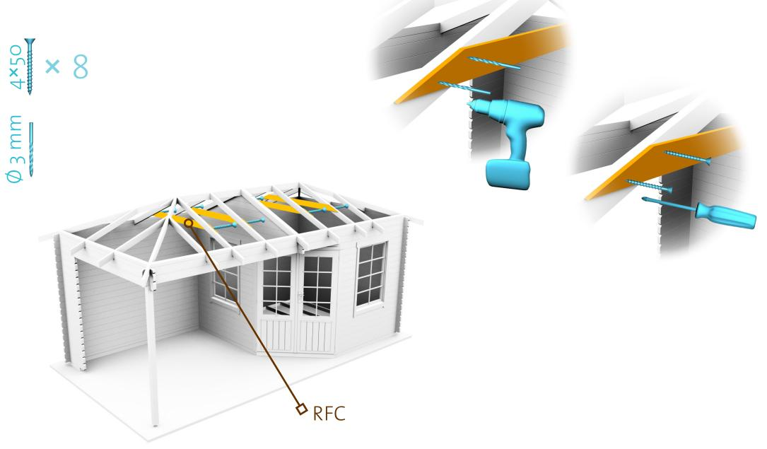
PLACE THE FIRST ROOFBOARD FLUSH WITH THE END OF THE PURLINS AND ATTACH WITH SCREWS
