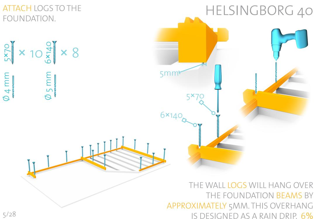
ATTACH THE NEXT ROW OF WALL LOGS INTO THE BOTTOM LOGS WITH SCREWS.
