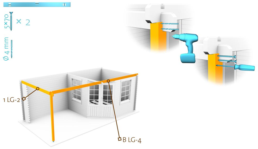
SCREW OUT THE SECOND PART OF THE POST FOOT SO THAT IT TIGHTLY TOUCHES THE GROUND.
